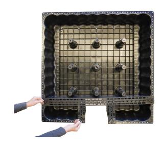
Push the CLEVA COMB™ firmly down into the grid securing the CLEVA COMB™ teeth into the CLEVA POD® structural grid and connect into the pre-drilled base flange using the CLEVA PLUG™s.
