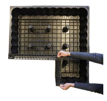
Measure and cut the CLEVA COMB™s to cover the exposed faces of the CLEVA POD®, push the CLEVA COMB™ firmly down into the grid securing the CLEVA COMB™ teeth into the CLEVA POD® structural grid and connect into the pre-drilled base flange using the CLEVA PLUG™s.
