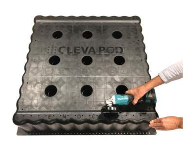
Cut the End Cap off following the pre-marked End Cap cut line and the section you wish to remove.
