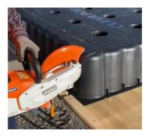
The Saw cuts cleanly through the CLEVA POD® and passes down through the cutting slots.
