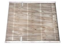
Measure 1020mm along both edges and cut two 30mm wide x 150mm long cutting slots into the cutting table.
